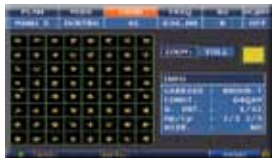
Constell. DVB-S2 = 8PSK, T & T2 = COFDM, C = QAM and all modulation parameters
